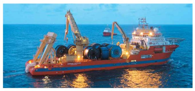
'Normand Installer' during the installation of flexible flowlines at the Okwori field offshore Nigeria
