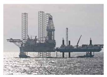
A jack-up drilling unit positioned next to the MOPU offshore Turkmenistan to drill two additional production wells
