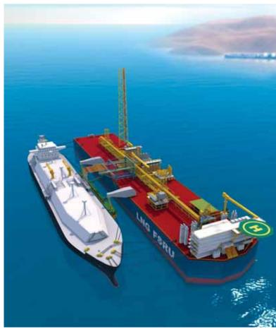
Large capacity turret moored FSRU with a discharging LNG carrier berthed alongside on a Soft Quay Mooring
