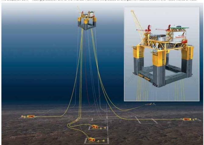
components necessary for deep offshore developments. The philosophy takes as a primary objective, to make such facilities quasi independent from water depth through the use of surface and near-surface technology. The reasoning is that equipment installed on the sea-bed in ultra-deep water is not only expensive in both capex and opex terms, but also faces technical difficulties with respect to accessibility and flow-control due to low temperatures.
