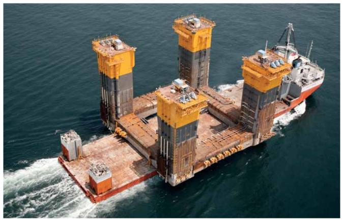
The hull of the DeepDraft Semi<sup>TM</sup> floating production system for the Independence Hub during dry transport from Singapore to the Gulf of Mexico
