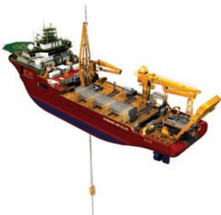
'Normand Installer' with the J-Lay system for SCR installation
